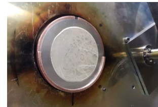
LN wafer temporarily bonded to an aluminum carrier via silver paste inside the implantation chamber
