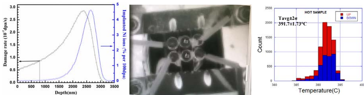
Displacement rate and implantation ion curves for 9 MeV \text{Ni}^{3+} in 316L SS (a), infrared image of irradiation stage with thin disk samples (b), and temperature histogram of the ion irradiation (c)
